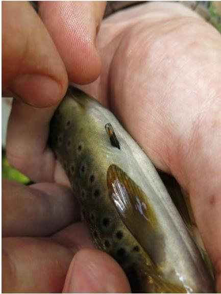
*Figure 16: Placement of a 12 mm PIT-tag in the abdomen of a brown trout. The placement of the PIT-tag in the abdomen meant that as little muscular functions of the brown trout were affected as possible. Furthermore, the PIT-tag would be closest to the bottom mounted antenna loop, increasing the likelihood of a successful registration upon passing the antenna.*
