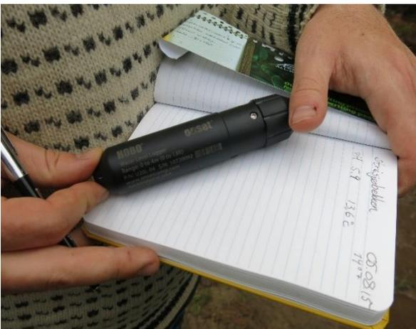
*Figure 12: HOBOT U20L, barometric pressure and water temperature data logger. This device was set to record water temperature and barometric pressure once per hour. This yielded an expected battery life of > 2 years. The device was placed under water and mounted to the water level gauge.*
