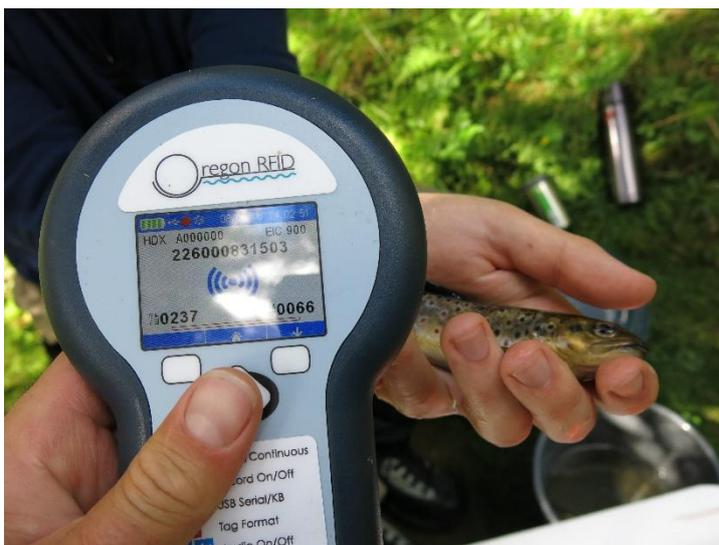
*Figure 17: Handheld PIT-tag reader. With the handheld reader, the number of the PIT-tag placed inside the abdomen of brown trout could be read. The long number on the display is the number of the PIT-tag.*
