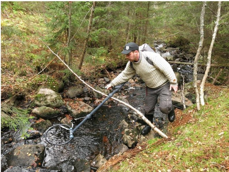
*Figure 15: Backpackreader operator in action. The portable antenna system is used to account for marked brown trout still residing in the tributary. The extended plastic tube, with a loop in the end is the antenna, while the registration system and batteries are carried in a small backpack.*
