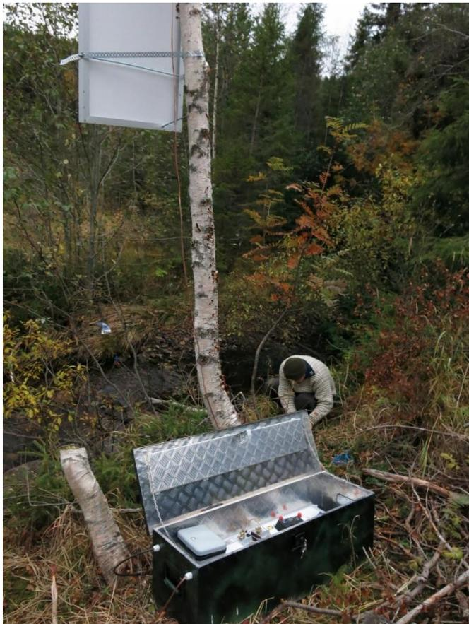
*Figure 13: Stationary PIT-tag antenna mounted at the inlet of a tributary to Lake Råsjøen. In the tree in the upper left corner of the image, is the solar panel, powering the station inside the aluminium box. Inside the box is the electronic components which register passing brown trout marked with PIT-tags.*
