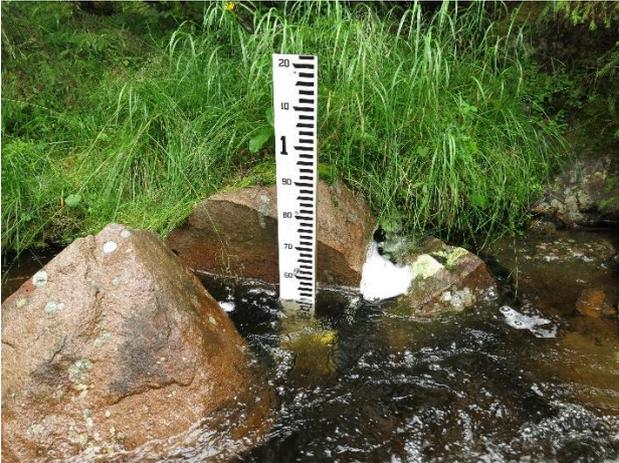
*Figure 11: A water level gauge was mounted in a small pool to have a reference point on water levels. The gauge was bolted into rock, to make it withstand floods and debris. The same equipment was mounted in each of the four tributaries.*
