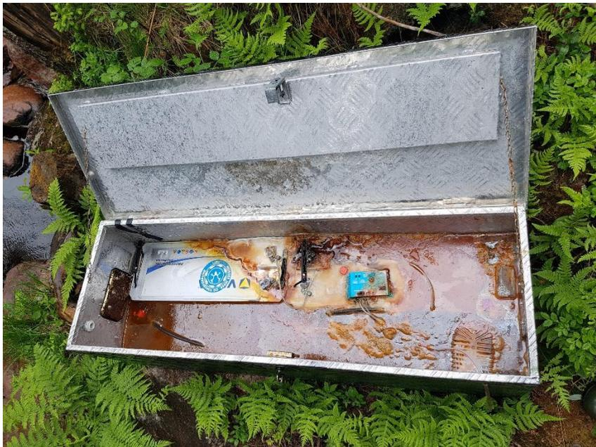
*Figure 38: A flood has filled the antenna station with water in tributary D in summer 2016.*
