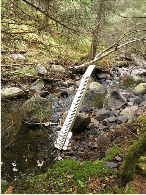
*Figure 39: Displacement of water level gauge and U20L logger after a flood in 2015, causing faulty temperature and barometric pressure data.*
