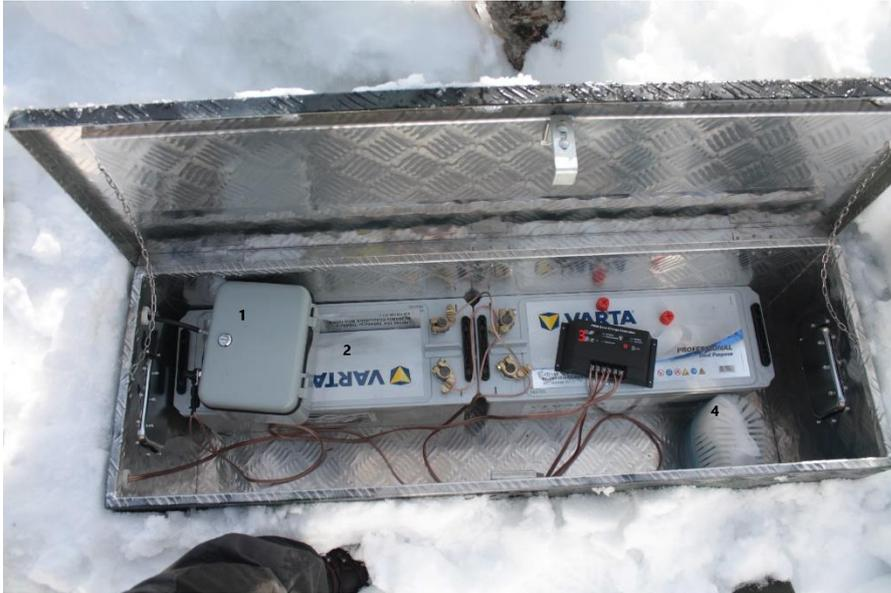
*Figure 14: The inside of the aluminium box containing the PIT-tag antenna registration station with the following components 1: PIT-tag registration box, 2: batteries, 3: Solar panel regulator box, 4: Dehumidifier to reduce humidity inside the box.*
